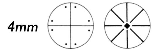
Consider the following three pairs of stereographic projections. Each of them correspond to a crystallographic point group isomorphic to **4mm**:
