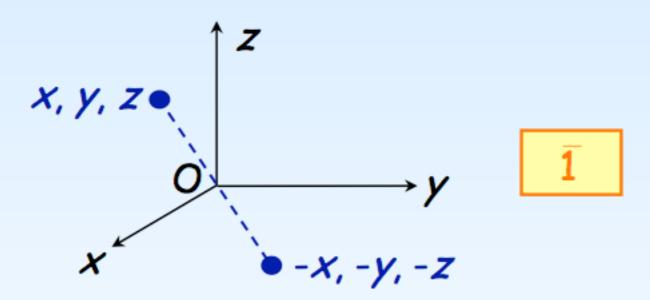
a crystal which has the inversion symmetry is called centrosymmetrical.
